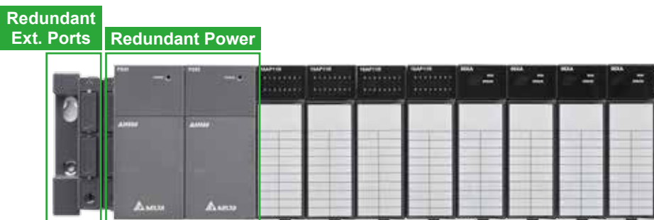
Redundant expansion backplane: AHBP06ER1-5A (6-slot), AHBP08ER1-5A (8-slot)
